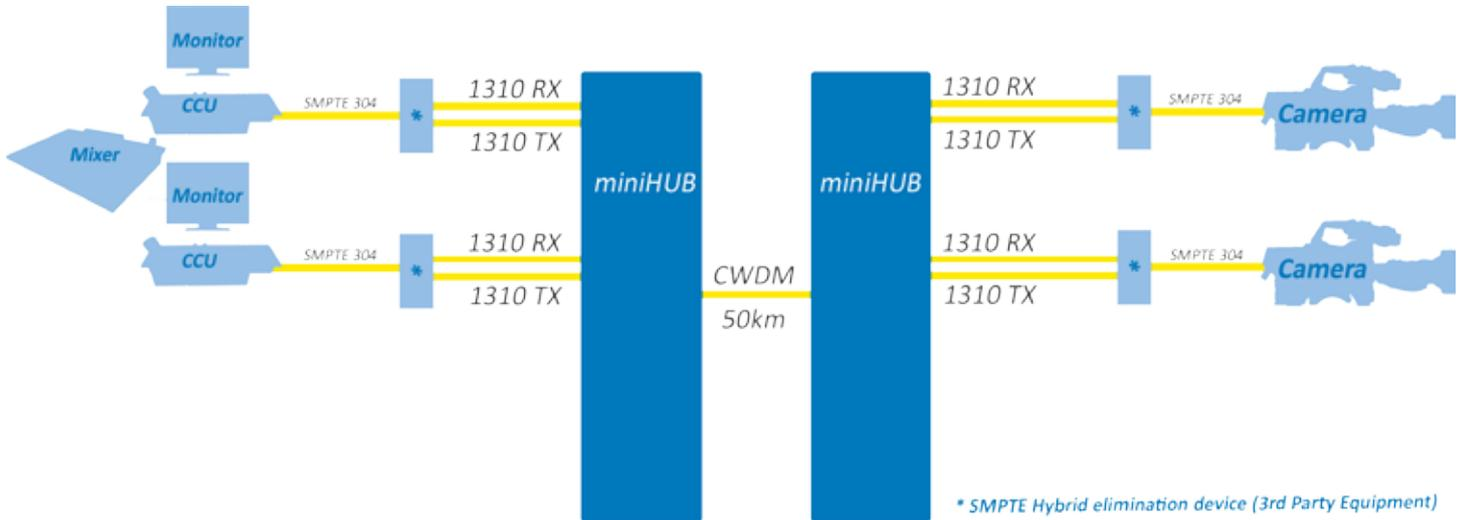
Optical camera based systems need to have conversion between SMPTE Optical connector to LC type optical connector and provide a power up sequence to enable the base station and camera communicate. Power is supplied from the SMPTE optical connector through the SMPTE Hybrid elimination device that powers the camera locally. This is the same for the CCU end of the camera chain.
